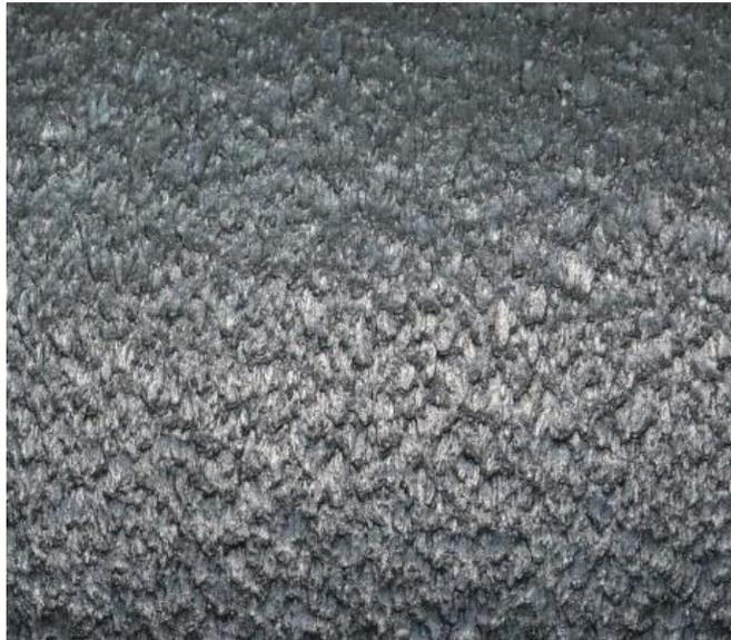
**Both LLDPE and HDPE are now available with a textured surface. Textured one side or both, texturing is an effective means of not only increasing the geomembranes' friction angle between the geomembrane and the backfill, it is also an important safety feature.**
